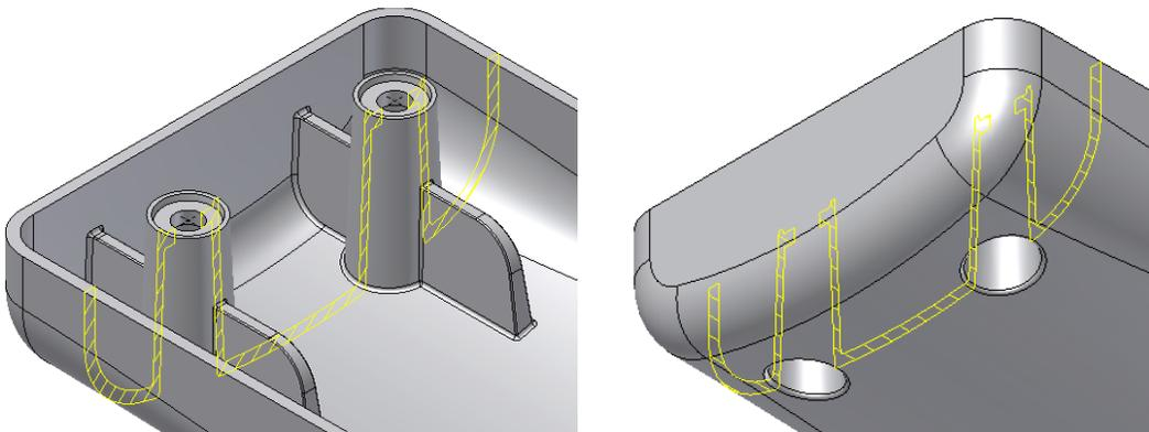
Build a Boss feature (thread component) on a part using On Point placement. Here the goal is to create a couple of thread bosses using one point from a sketch and one 3D work point, for instance in order to have different boss heights.
