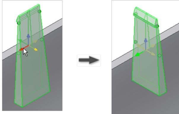
**Work points** or **sketch points**, select placement points from different sketches or work points, in this case the sketch normal is not used, and the beams direction and hook/catch direction must be defined by selecting geometric or work elements.
