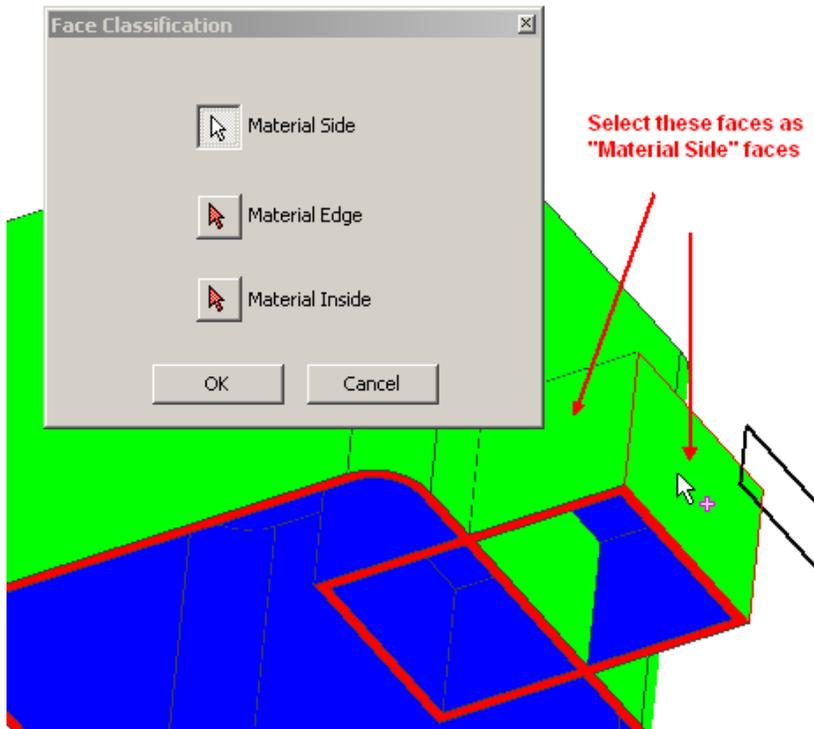
The, the Join To Shell extrude produces the expected result:
