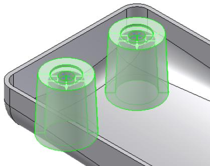
6. Adjust the Boss head parameters or use the manipulators until the desired dimensions are reached.
