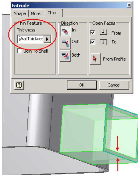
This value controls the thickness of the thin feature being created. The default value is always “WallThickness”, which is a parameter that is set in the Wall Properties command for the part. It can be overridden for each feature, if desired.
