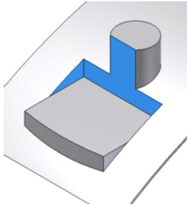
The extent of the **platform** wall is by default "Through all" which means that it is extended to the next face of the target body.
