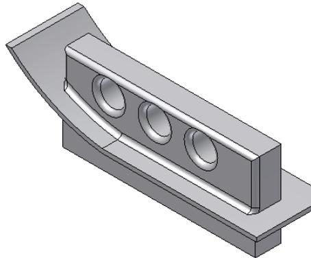
Against features, only the edges generated by the source selected faces and the faces of the features in the scope selection set are filleted, for instance consider the three holes to be in the scope selection set.
