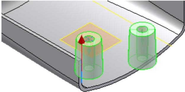
7. Make sure that the bosses can extend to the target body, i.e. their projection will be completely within the part body boundary.
