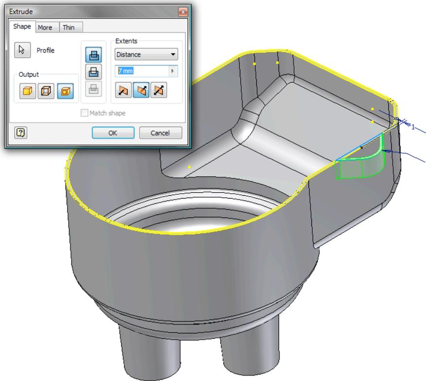
46. On the Thin tab, ensure that only the “From” face is open and hit **OK**.
