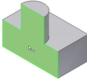
When doing a Rule-based fillet, “Free Edges” rule, with the cylinder in the Source set you get this result for **Remove Merged Faces OFF**:
