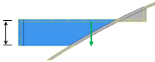
To Surface specifies the surface to extend the platform walls to.
