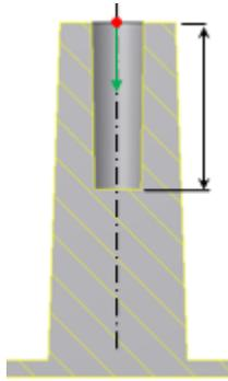
**Full Depth** the hole is automatically extended to the internal wall face, this is the best practice to avoid sink marks in molded plastic parts.
