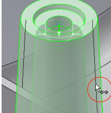
7. Add 2 stiffening ribs, make sure they are oriented like in the picture (it may be necessary to enter 90° angle depending on the sketch Y axis orientation). Adjust the ribs dimensions using the manipulators or the dialgo input fields.
