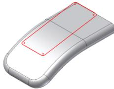
2. **Island:** an area filled with material usually at the center of the grill. The island often has the same thickness as the shell. It must be a closed sketch.
