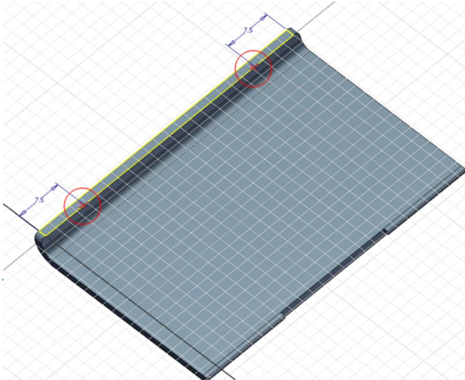
2. Build a sketch on the wall narrow face as indicated in the picture. Make sure you have the internal edge projected since the positioning points should stay on this edge to make the Snap Fit face flush with the internal face of the bottom solid.
