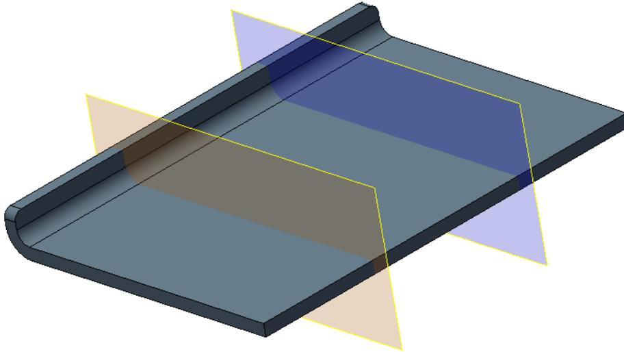
3. Build two work planes parallel to the side faces of the battery cover at 15 mm offsets
