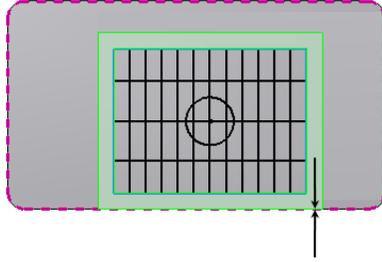
The boundary sketch is the only mandatory element to build a Grill. The area of the openings of a Grill feature is reported in the Flow area section of the dialog box and in a Reference parameter. The flow area does not take into considerations the optional draft angles.
