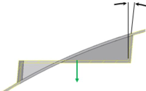
Clearance Taper Specifies a draft angle for the clearance walls.
