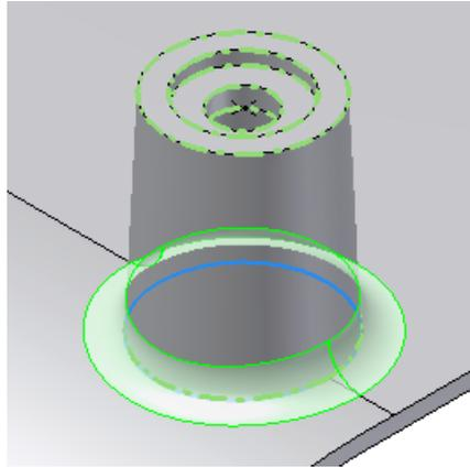
4. “Click to add” another rule. Set the Source to “Feature” and select the same Boss. Set the Rule to “Against Part”. This time uncheck the “All Fillets” toggle. Enter a radius which is equal to the one entered in the rule above augmented by the part thickness.
