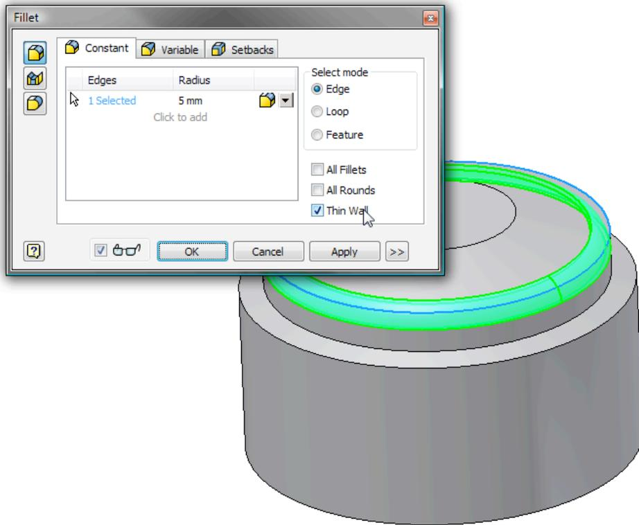
15. The fillet is created on the edge selected with a radius of **5mm** and... the matching inside edge is filleted automatically to a radius of 5mm – “WallThickness.” (Note: Wall properties also have radius values for Outer Radius and Inner radius. You could use these named parameters as well).
