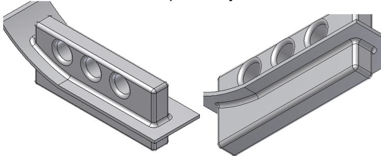
Against Part, only the edges formed by the faces of the features and the faces of the part body are filleted.
