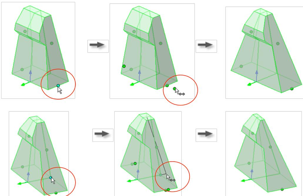
1. Profile manipulators, to define the linear parameters of the snap-fit.
