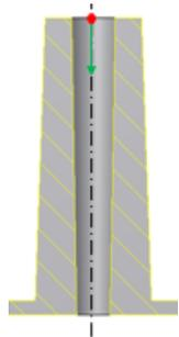
If the **hole check mark** is **off** the thread boss can model an ejector pin
