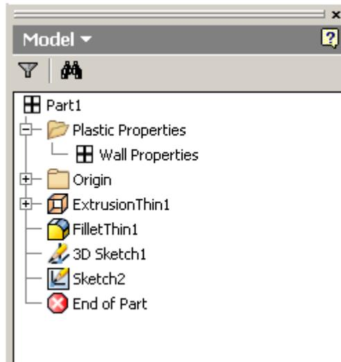
The Inventor part browser contains a new Folder node: “Plastic Properties”, which contain the wall properties for the plastic part. Additionally, any “thin wall” features will be shown in the browser using a different icon than standard Inventor.
