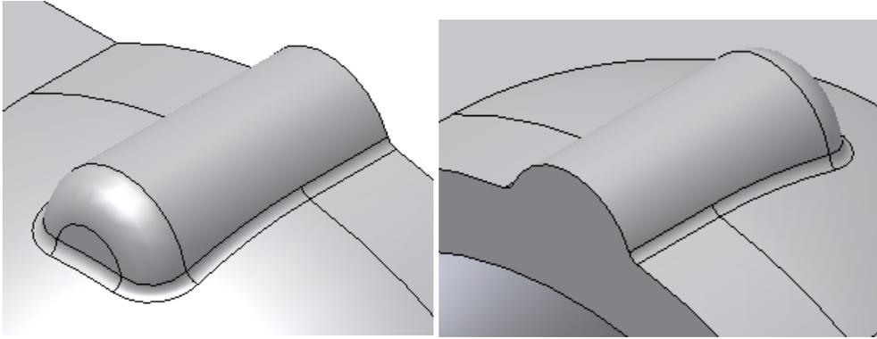
How to model constant wall thickness between a Boss and a part body.
