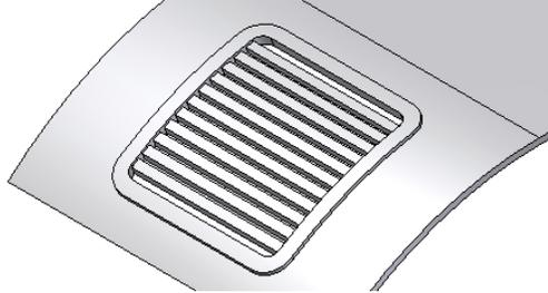
2. Click the Rule based Fillet tool of the Plastic Features panel bar.
