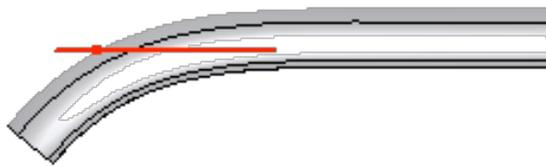
2. Build a 2D sketch that is on either sides of the thin-walled part
