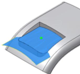
The **clearance** walls extend above the landing area cutting material across the entire target body.
