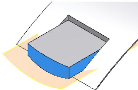
Offset specifies an offset from the reference surface in the To Surface option.
