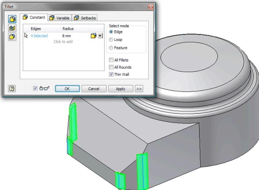
29. Notice all the thin features keep constant wall thickness even though the geometry is getting more and more complex.
