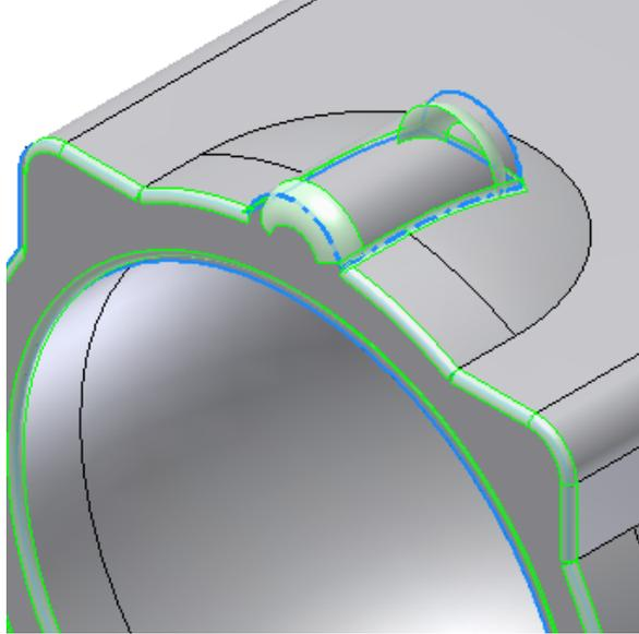
13. ... to avoid the merged faces to be included in the edges selection click on the “More” button and check the “Remove Merged Faces” toggle. The preview fillets on the planar face disappear.
