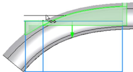
The landing area can also coincide with a surface (“To Surface” option on the More tab).
