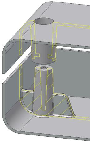
The Boss feature provides for the design of both components of a fastener placement, called **head** and **thread**, in addition it allows the design of fastening ribs that often occur especially when the length of the boss is greater than three times the diameter.
