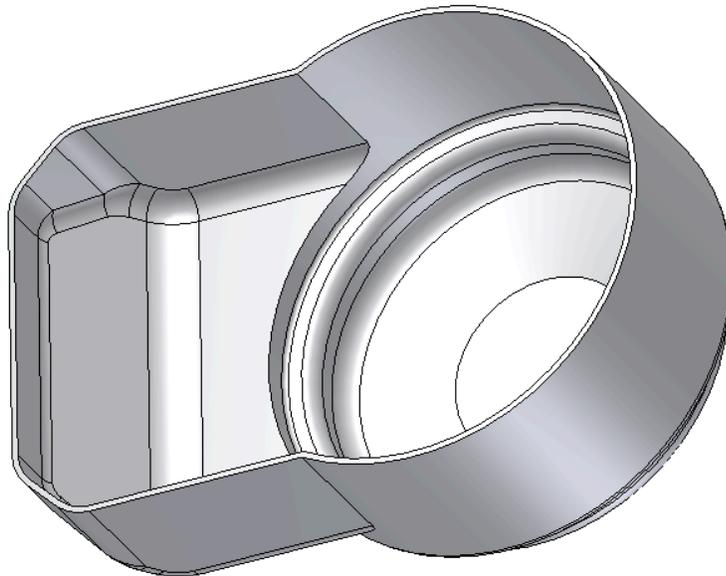
33. To continue we need a construction plane. From the Molded Features panel bar select the **Work plane** command.
