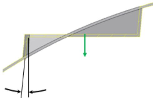
Landing Taper Specifies a draft angle for the platform walls
