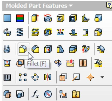
14. Notice the new thin wall check box. Select the edge shown and enter a fillet radius value of **5mm**. Hit **OK**.
