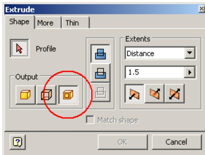
If this output option is selected, it enables creation of “thin extrude” features, which is the primary Extrude enhancement in the Plastic Environment. If this option is selected, options on the Thin tab become enabled.
