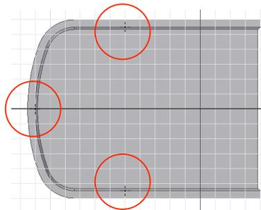
3. Click on the Snap fit tool of the Plastic Features panel and make sure that the Placement method is “From sketch” and the Snap fit style is “Cantilever Snap Hook Join”.
