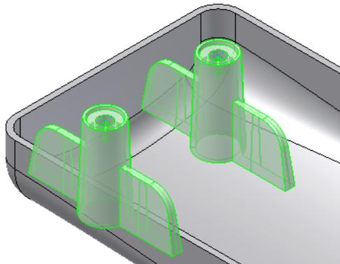
8. Add fillets at the intersection boss-body, at the ribs edges and at the intersection ribs-boss. Hit OK, the mounting Boss is done.
