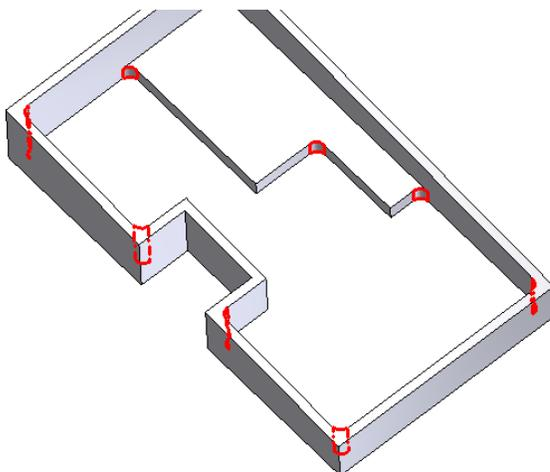
**All Rounds** option: Convex edges. For example, in the incident edges rule above the All Rounds option would filter the edges as indicated.
