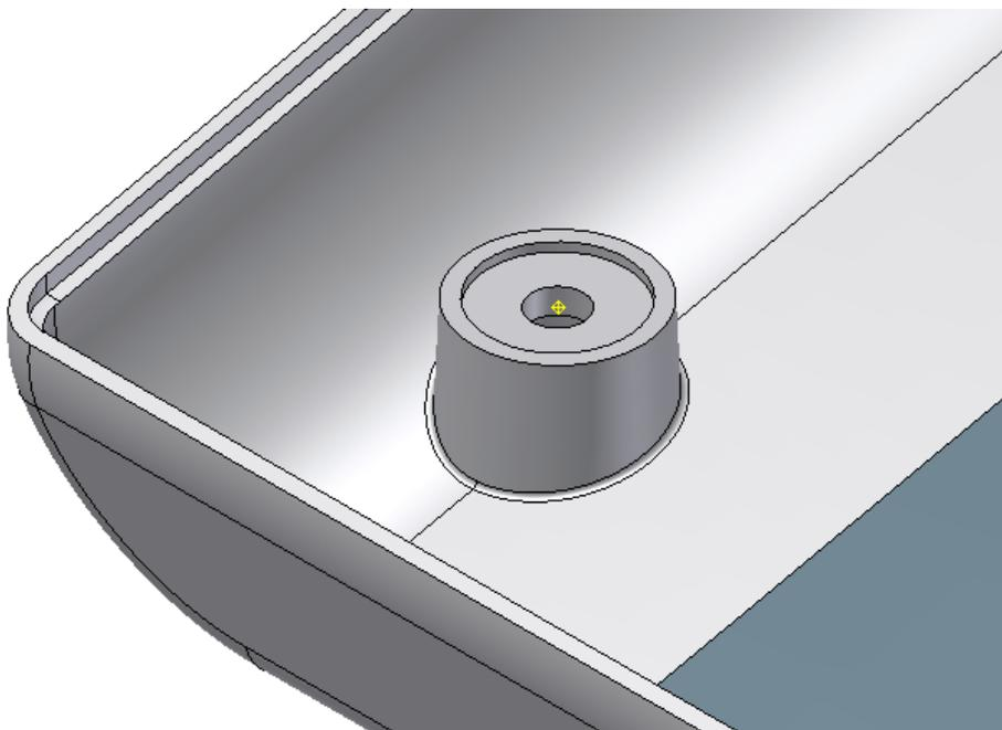
We now build the mating bosses for the thread part of the fasteners on the top.
