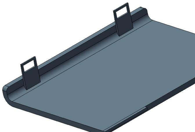
We now want to fillet the edges at the intersection between the Snap Fit and the battery cover solid. A **Rule Fillet** can do the job.
