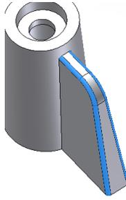
**Rib blend radius** at the intersection between the ribs and the boss.
