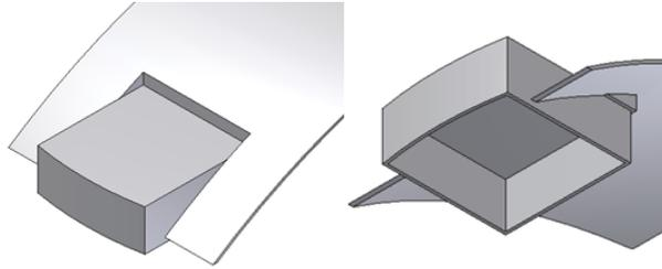
To correct this geometry, use the “To Surface” option on the Shape tab or change the extent parameter for the platform wall to be flush or higher than the body boundary.
