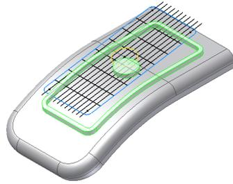
6. Select the Rib profiles. You can use window selection (by dragging the cursor left to right you select only what is entirely included in the window, by dragging the cursor from right to left the window selects whatever entities are intersected by the window boundaries). Enter the Rib Thickness, Height, Top Offset (from the Grill Boundary face) parameters.
