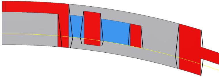
Alternatively, you can define the parting element as the part surface (before the application of the Grill) at a given Offset from the Boundary outside face. By changing the offset amount, you can position the parting element where deemed necessary. The outside faces remain neutral.
