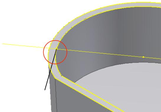
2. Build the construction elements and a 3D work point on the internal wall edge at the position where the Snap fit is desired, for instance the *3D work point* can be the end of a line that is tangent to the internal edge and the hook direction can be a work axis defined by the 3D work point and the center of the circular edge.
