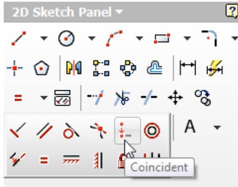
20. Create a coincident constraint between the midpoint of the short edge of the rectangle and the center point of the circular faces of the part.
