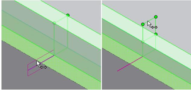
7. Expand the Path Extents selector and select the two planes and the two points. At first the Lip algorithm makes a tentative choice of sectors. Use the green and yellow dots to customize the sections to keep or remove
