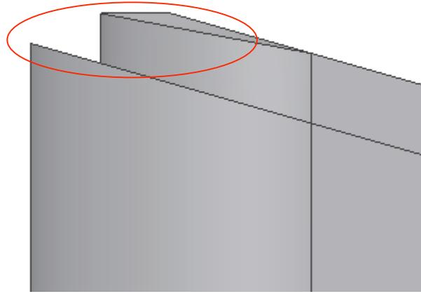
11. If necessary, you can correct it by cutting the part at an offset of the parting element (See the red profile).
