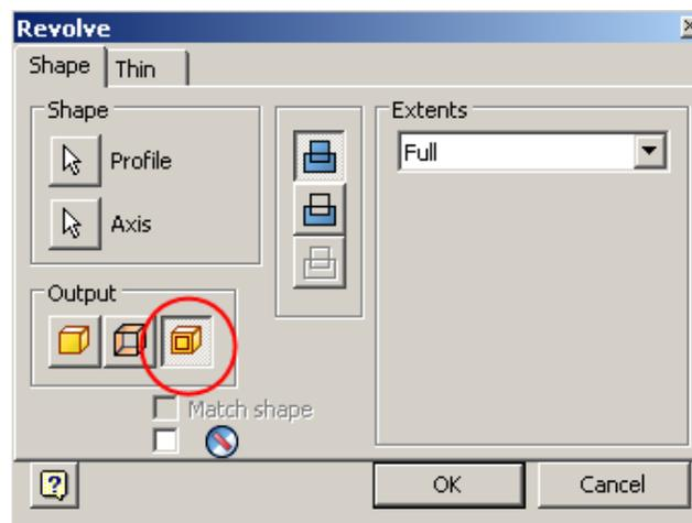
If this output option is selected, it enables creation of “thin revolve” features, which is the primary Revolve enhancement in the Plastic Environment. If this option is selected, options on the thin tab become enabled.
