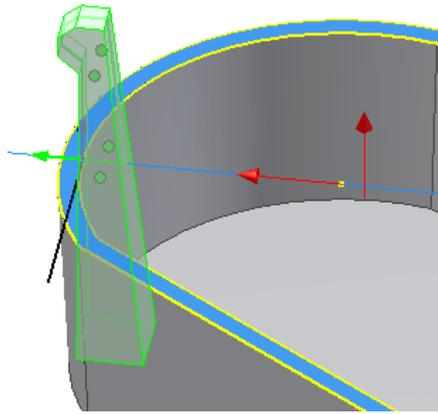
5. Adjust the shape parameters as desired and click OK.
