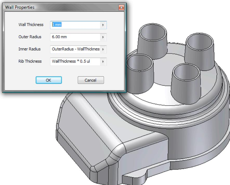
3. Change the wall thickness to **1.5mm** (Note: larger values will not work as we have created small internal fillet values that will begin to be consumed and cause errors. This is a limitation of this technology preview)
