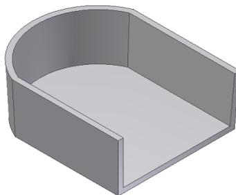
1. Create or import a thin walled part. The goal here is to place a Snap fit feature on the circular edge at a position that is not convenient for the “on sketch” positioning style, for instance at a point on the edge where the hook direction is not likely to be aligned with a sketch X or Y axis.
