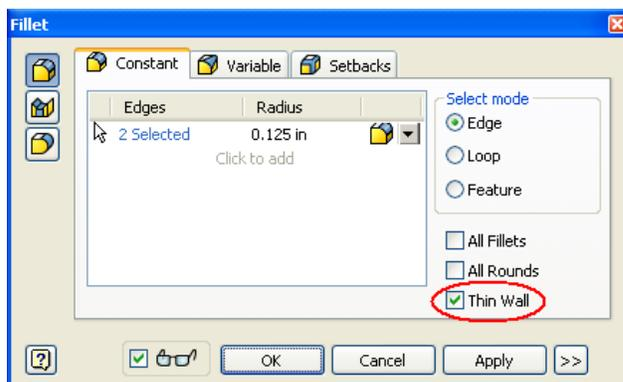
If the 'Thin Wall' checkbox is clicked, the resulting fillet will be thin-walled i.e. the corresponding opposite edges will also be filleted.
