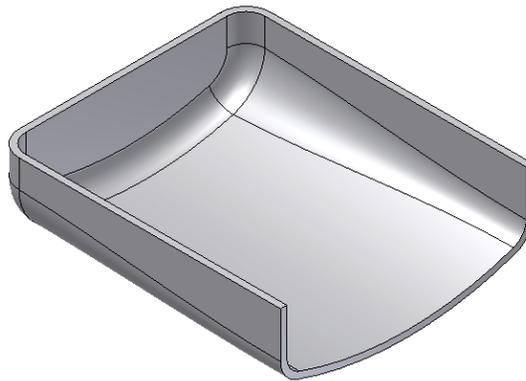
2. Build the construction elements: one sketch point and one 3D workpoint where the Bosses are desired.
