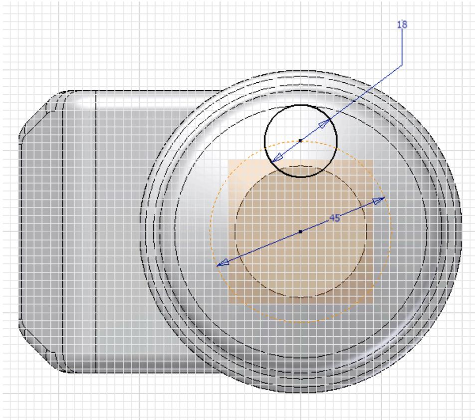
36. Create an Extrude feature and enter a distance of **30mm**.
