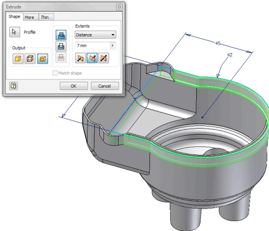
53. On the Thin tab, ensure that only the **“From”** face is open and hit **OK**.
