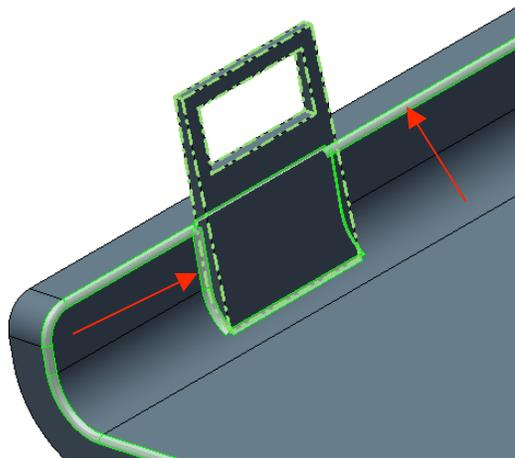
14. We do not want the fillet around the top edges (red arrows) The edges where included because they share the curved face of the Snap Fit that coincides with the curved face of the battery body (they are called “merged faces”), we can simply skip such merged faces (and all the edges they share)
