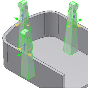
6. Adjust the beam and hook parameters or use the manipulators until the desired shape is reached. Note that the shape manipulators are not active when the Hook direction is down (to facilitate the selection of the directions) .
