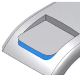
The rest feature is based on a sketch that defines the **landing area** boundary. You can drag the position of the landing at offsets of the sketch plane.
