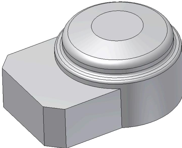
27. Add a second chamfer. Use the “Distance angle” construction option and enter a distance of **20mm** and an angle of **35**. Hit **OK** when ready.
