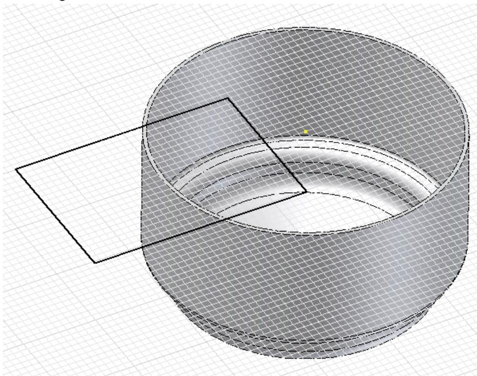
19. From the 2D Sketch panel bar select the **Coincident** constraint from the constraint fly out.
