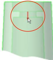
It has to be noted that the feature can only exist if it can be extended to a face of the target part body that is opposite to the placement point in the boss direction. The feature determines automatically the closest face of the part body it can extend to, users can select a different target body and flip the direction as well.
