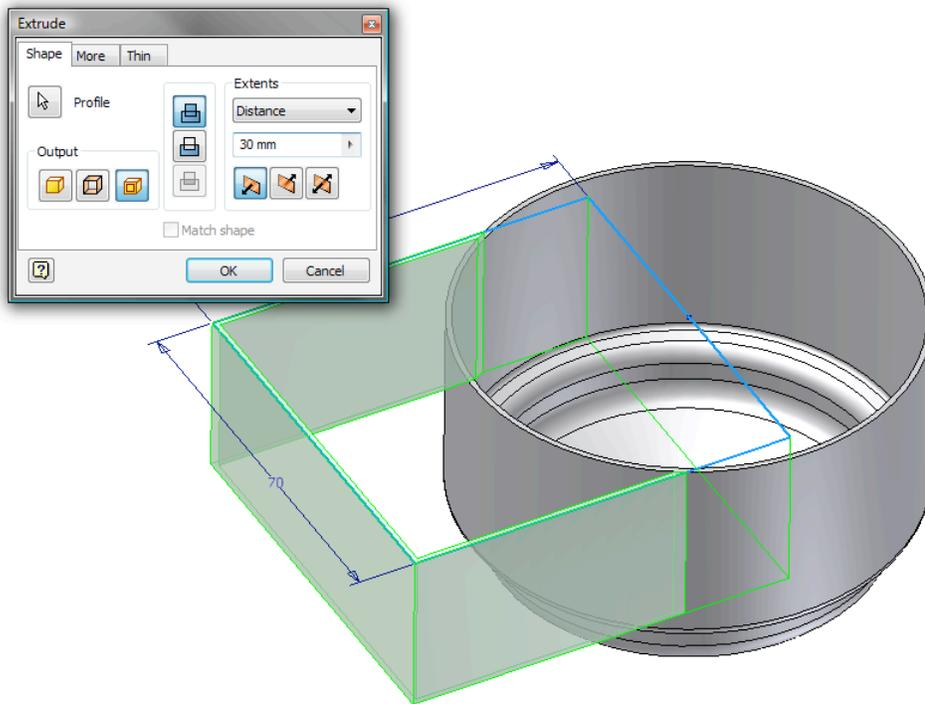
24. Switch to the **Thin** tab and uncheck the “**To**” check box for Open faces. Experiment with these settings to see the results of the preview. Also notice that in the thin features frame there is a new option for Join to shell. This allows you to shell as you go! Be sure to set your options shown before proceeding, and then hit **OK**.
