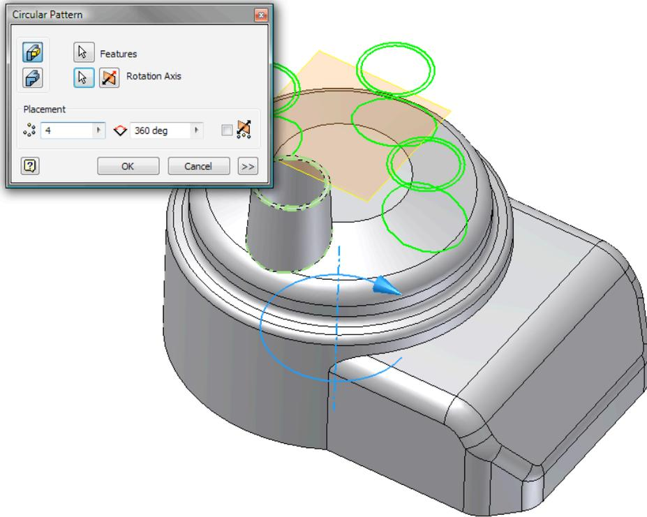
42. Even the new patterned features automatically join to the shell and part still has constant wall thickness.
