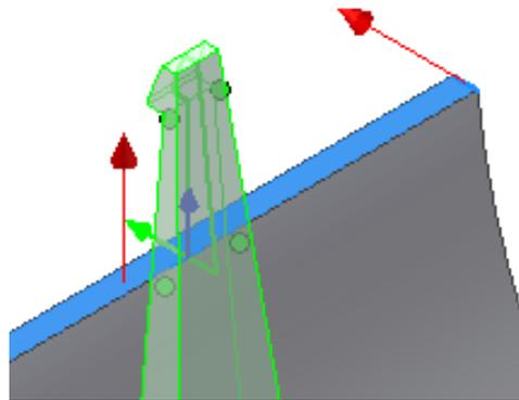
Once the beam and hook/catch directions are chosen the user can still flip the orientation of both by selecting and dragging the arrows.
