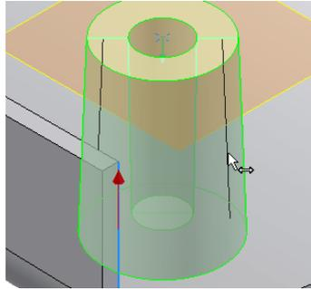
9. Stiffening ribs are not necessary here, hit OK, the Boss is completed.
