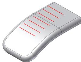
For the Grill feature to be successful the boundary external contour projection (plus a 10% tolerance band around the external contour) must stay entirely within the part surface and no material gaps (holes) are allowed inside the boundary projection. Examples:
