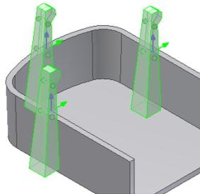
5. Notice that the four possible directions for each Snap fit are aligned with the X Y axis of the sketch plane. Click on the hook direction arrow to properly orient each hook.
