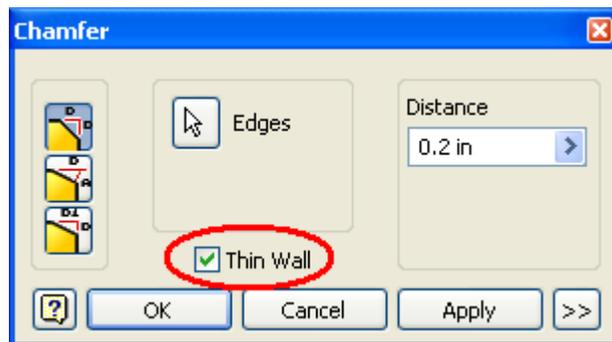
If the 'Thin Wall' checkbox is clicked, the resulting chamfer will be thin-walled i.e. the corresponding opposite edges will also be chamfered.
