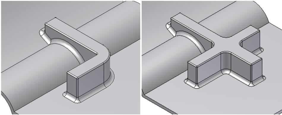
Supported are also drastic topological changes of the feature involved in the rules. For example, a redefinition of the extrusion profile rebuilds the rule-based fillet without any further interaction.
