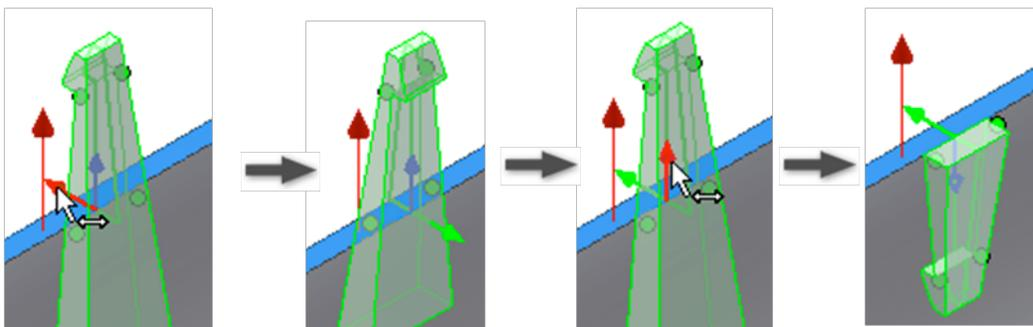
Finally the user has the option to automatically extend the shape of the beam until the next face.
