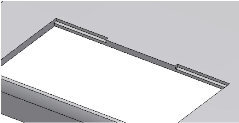
26. When placed in an assembly the Lip and Groove will mate as pictured.
