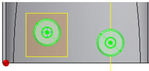
8. Adjust the dimensions as usual, and assign a fillet for the intersection boss-part body.
