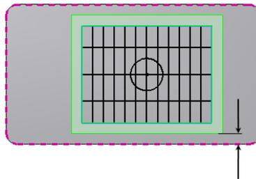
Grill will not compute, the external contour of the Grill boundary projection is not entirely included within the target body.
