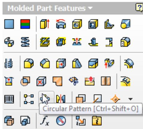
41. Select the last feature to pattern and use any circular face from the first revolve feature for the rotation axis. Enter **4** for the pattern count. Hit **Ok**.
