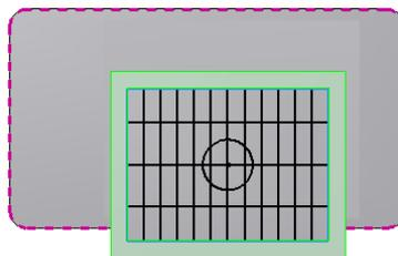
Grill will not compute, the external contour of the Grill boundary projection is too close to the margin of the target body (the distance tolerance is below the 10% threshold).
