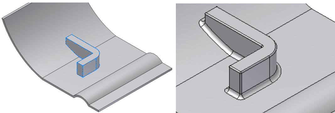
You can make this fillet with a single rule-based fillet on the highlighted feature with two rules: **Free Edges** (meaning the edges of the feature itself) and **Against Part** (meaning the intersection edges feature-part). Each rule requires only the selection of the feature (so two feature selections total), each rule can have its own radius.
