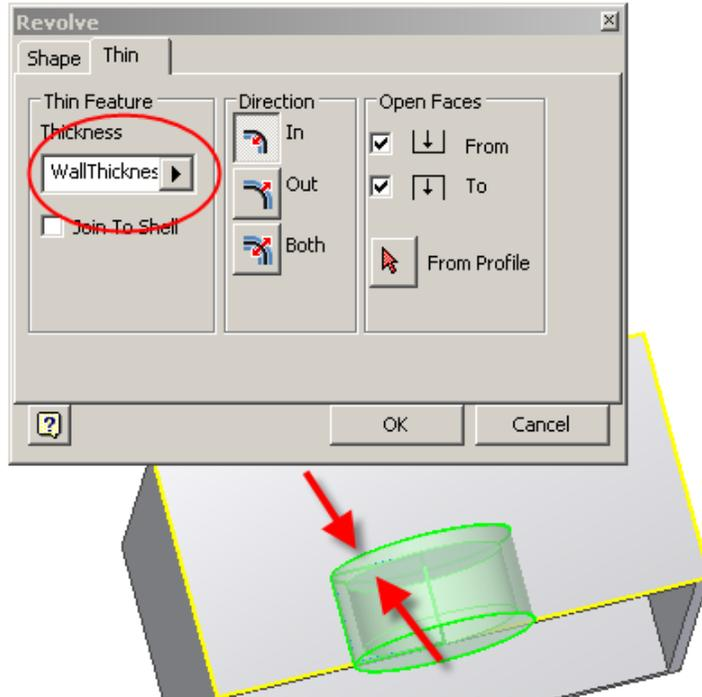
6. This value controls the thickness of the thin feature being created. The default value is always “WallThickness”, which is a parameter that is set in the Wall Properties command for the part. It can be overridden for each feature, if desired.
