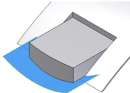
It is possible to specify a draft angle for both the platform and landing walls.
