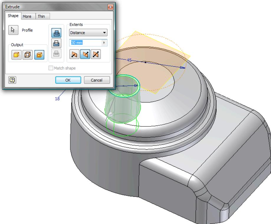
37. Switch to the **More** tab and enter a draft angle of **3deg**.
