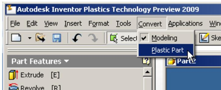
3. This process can be used to either convert a part designed in an earlier release of Inventor to a Plastic Part, or to convert a new part opened with the “Standard.labipt” template into a Plastic Part.
