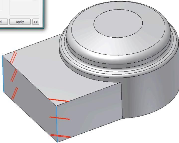
26. Notice that the chamfer is automatically created “thin” like the fillet.
