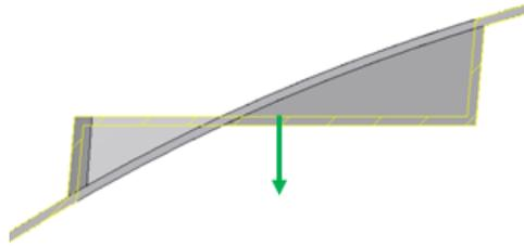
**Tip:** If the Rest boundary projection along the sketch normal does not stay entirely within the target body, the feature ends up extending the platform walls also inside the body.
