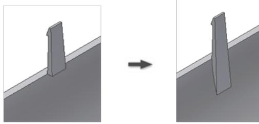
The *dimensions* of the Snap fit feature can effectively be set by use of *manipulators* that are available on the preview to interactively define the geometric parameters when precise dimension input is not used.
