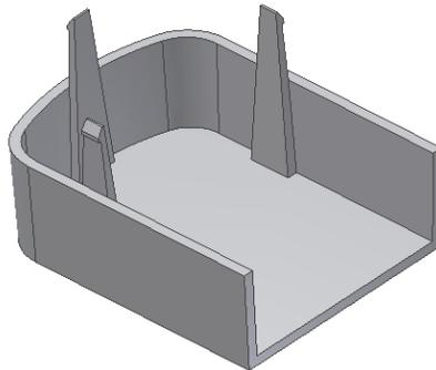
Build a Snap fit feature on a part starting from a 3D point.
