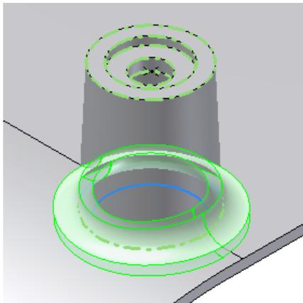
5. Click OK, the Rule fillet is done and the part has a constant thickness at the intersection Boss-part body.
