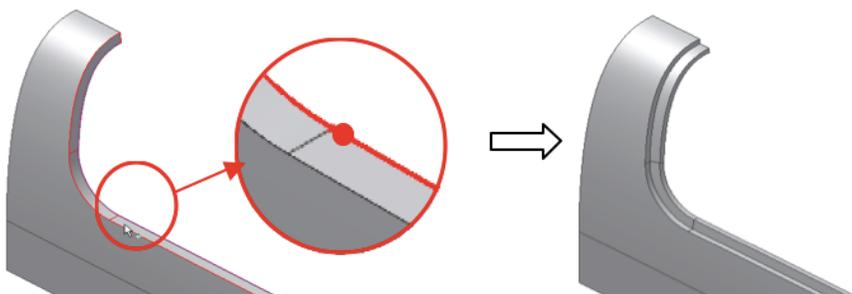
Alternatively, the Lip/Groove may be referred to a Pulling direction. In this case, the Lip/Groove cross-section stays parallel to the selected pulling direction along the entire path.
