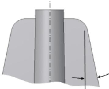
**Start angle** it's the first rib inclination angle with respect to the sketch Y axis (when Placement is On Sketch), or with respect to the projection of the start direction on a plane normal to the Boss direction (when the Placement is On Point).
