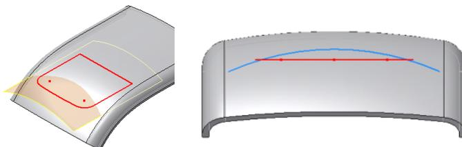
3. Build a surface that spans over the entire sketch in the position where the landing surface is needed.
