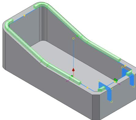
6. Use the manipulators on the preview to adjust the Lip cross-section and the clearance volume. Note: You can drag the cross section to a more convenient location along the path.
